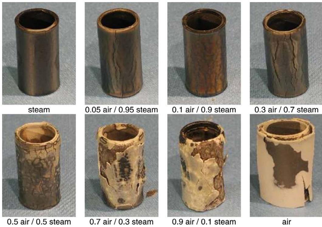
Fig. 10. Post-test appearance of specimens oxidized at 1200 °C in mixed air–steam for 1 h.
